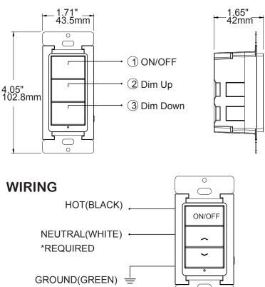
\* Switched Hot to Load is not required. Switching is done at the power pack or in-fixture load controller.
